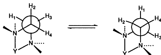
Fig. 6 Ethylenic inversion in yttrium complexes
